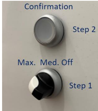
Ilustración 5. Temperature selection button and temperature confirmation knob of ADAMO robot
