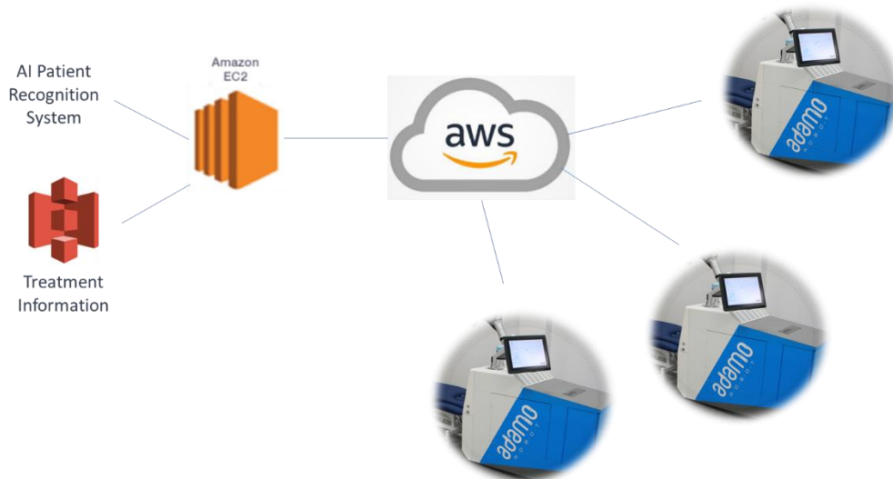
Illustration 3. Adamo robot: architecture SW in the cloud.
