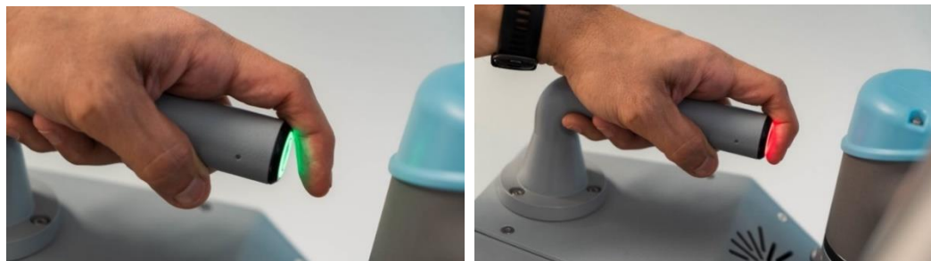
Illustration 39. The change in colour of the handle button of the robot in order to fix the necessary points.
